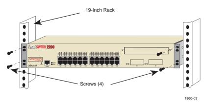
Figure 3-4 Installing the 2E4X-27 in a Rack
